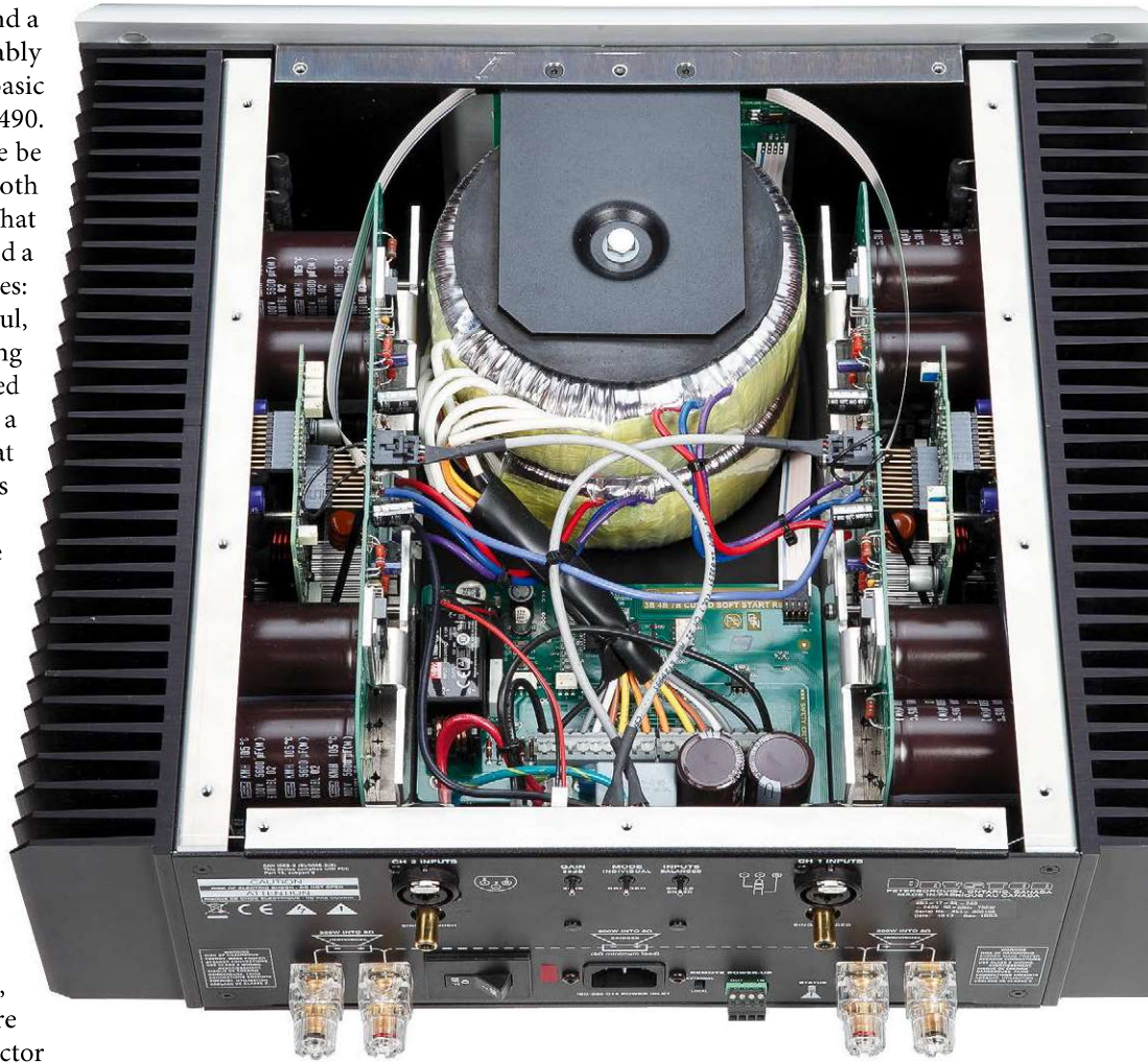
▲ Two stacked and solidly clamped toroidal core transformers contribute to the hefty weight of the 4B3.
